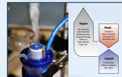
Figure 3. Heat generated by the heating element and the cooling influx of water allow thermal equilibration.
