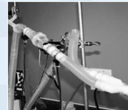
Figure 4. Setup of C-Force™ [proto-type model in ventilator circuit proximal to the 'wye'.
